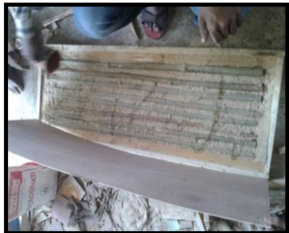
Fig 8(e): Preparation of Bamboo Panel
