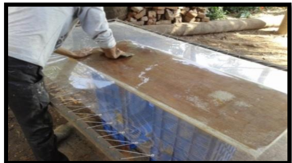
Fig 8(l): Preparation of Bamboo Panel
