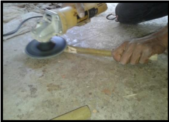
Fig 8(b): Preparation of Bamboo Panel
