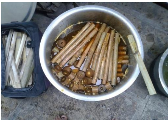
Fig 3: Dipping Process of Bamboo
